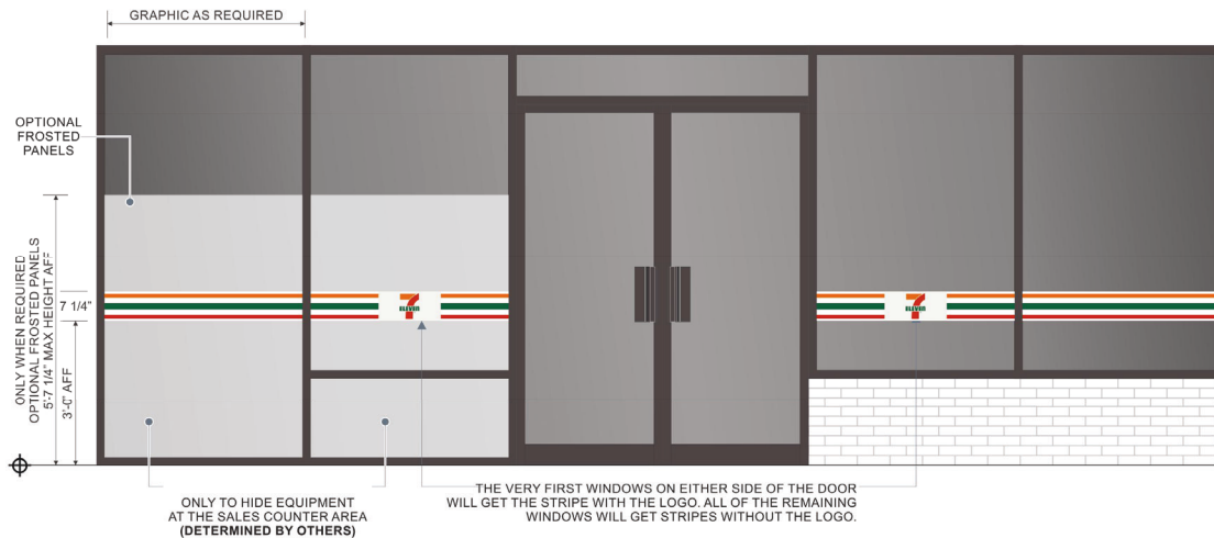
Front Elevation & Side Mounting Detail - ATM S/F Window Sign - Sign D NTS
